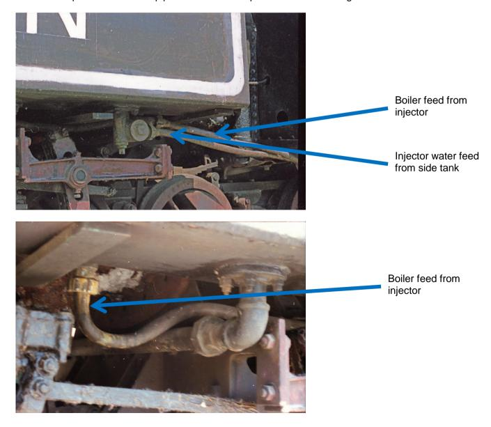
The discharge clack valve was fitted inside the boiler about half way along. It looks like the feed from the tank incorporated an isolation valve presumably to enable injector maintenance without having to empty the tanks.
