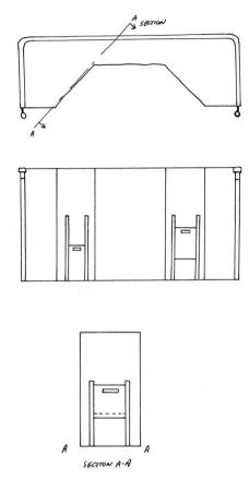
This is also based on a photo of the GVT Baldwin on page 182 of John Milner's Rails to Glyn Ceiriog (part 2) book where the angle of the photo suggests a frame for the coal door on the angled side of the bunker.
