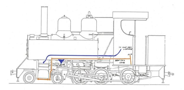
DAIN LOCK LEVER & LINICASE ON DRIVERS SIDE C.R. RHS OFLOCO WHEN LOOKING FORMARD FROM CAB) LEVER PROTED NEAR TOP OF CYLINDER WITH CROSS ROD TO LHS AT ROTTOM.
