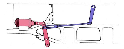
The steam brake cylinder and brake block operating arm are shown in red while the hand brake link and central pivot arm are shown in blue.
