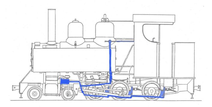
Each pair of brake blocks was joined together at the bottom by a cross-rod (the blue dot in the diagram below). According to my sketched notes from the brief inspection that I got of Lion, the centres of each cross rod were joined to each other (the red lines) with off-set links (the black lines) a bit like this:
